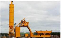
YHZS25 Mobile Concrete batching Plant basic performance parameters
